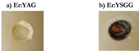
Fig. 9: Pictures of cavities in dentin, made with Er:YAG and Er,Cr:YSGG lasers following three consecutive laser pulses of the same laser pulse fluence of 80 \text{ J/cm}^2 [19]. In order to eliminate any influence of the difference in pulse duration, the Er:YAG pulse duration was adjusted to match that of the Er,Cr:YSGG (Waterlase PFN S mode). In this experiment, no water spray was used.
